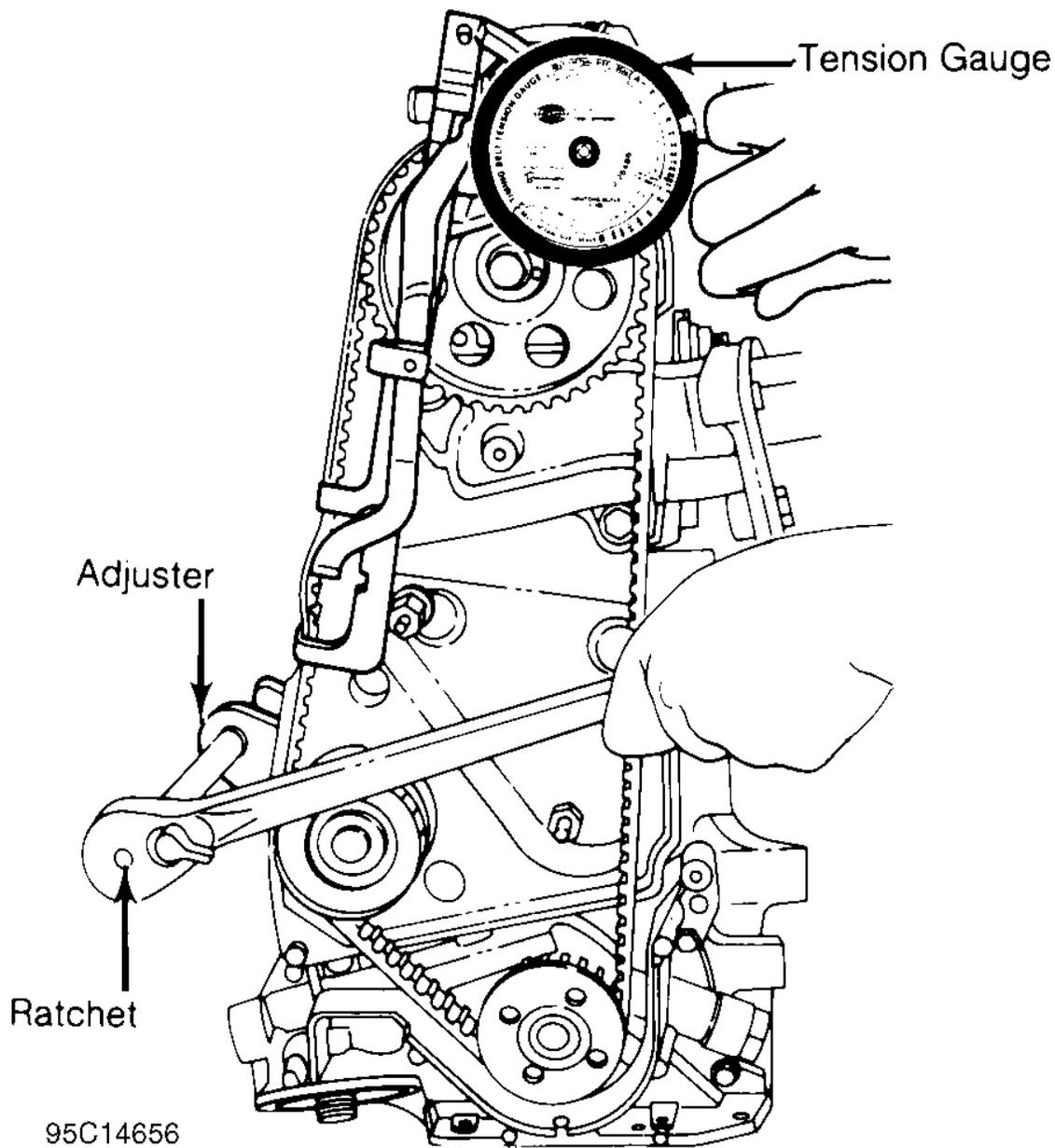
**Fig. 26: Adjusting Typical Timing Belt Tension**
