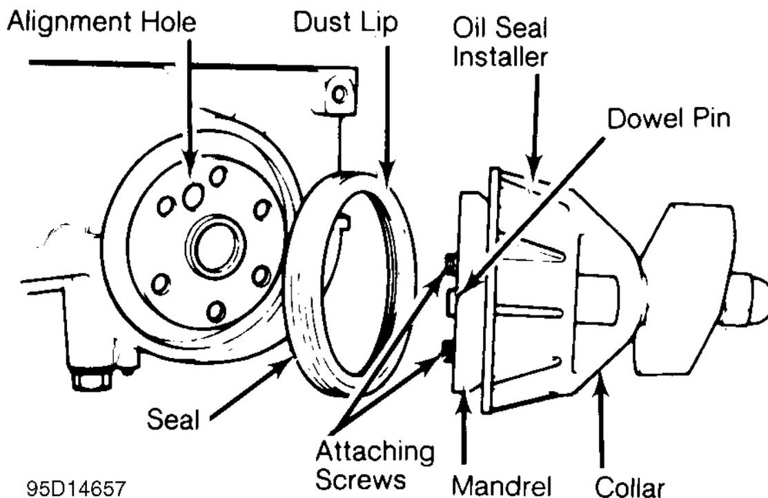
**Fig. 27: Installing Typical One-Piece Oil Seal**
