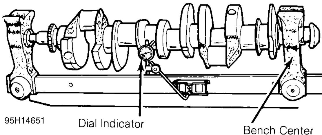
**Fig. 21: Measuring Crankshaft Main Bearing Journal Runout**
