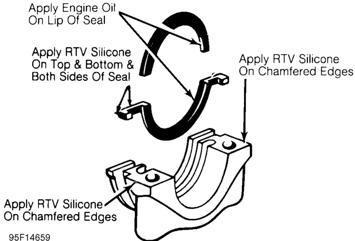
**Fig. 29: Installing Typical Split-Rubber Seal**
