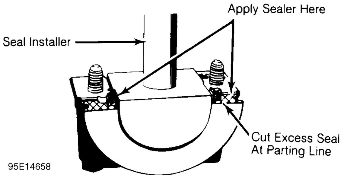
**Fig. 28: Installing Typical Rope Seal**
